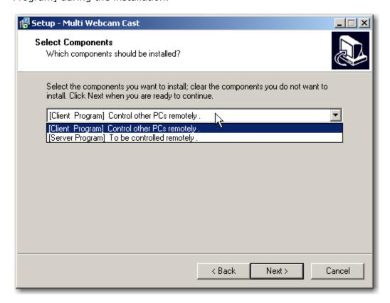
In the meanwhile, you need to run <u>multi-webcam-cast setup.exe</u> on the computer that you want to control/monitor remotely. When installation goes into "Select Components", select the [Server Program] option.
